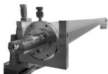
High Powered Hollow-Core Fiber Compressor
